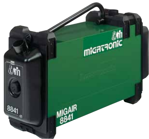
MigAir 841 * MigAir 841 is equipped with an automatic start/stop function connected to a holder on the extraction unit. Once welding has started, extraction will start. The stop function is adjustable with 5-25 seconds delay so as to ensure that all fume is extracted. At the same time the torch is additionally air cooled. The automatic stop function is energy saving and ensures a longer life of the MigAir 841. Equipped with indicator for replacement of no-touch filter. 220 V. Article no. .... 82031011
